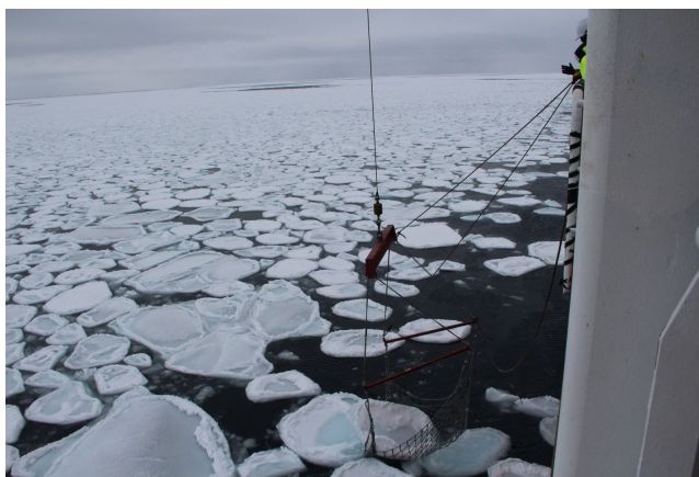
Figure 4. Sampling of solitary pancake ice floes with diameters of about 2.5 m using the ship’s crane.
