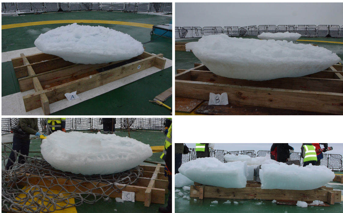
Figure 5. Pancake ice floes placed on wooden grids on the ship's helideck: Pancake A (top left), Pancake B (top right), Pancake C (bottom left) and Pancake D (bottom right) shattered into six large pieces during removal from the net.
