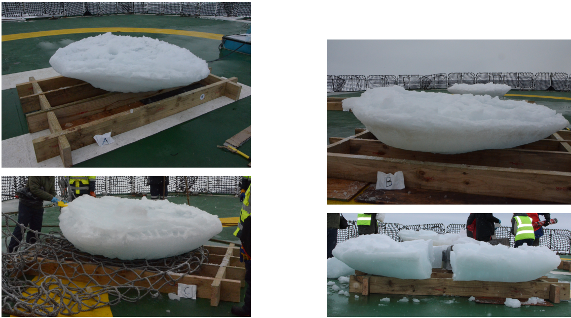
Figure 5. Pancake ice floes placed on wooden grids on the ship’s helideck: Pancake A (top left), Pancake B (top right), Pancake C (bottom left) and Pancake D (bottom right) shattered into six large pieces during removal from the net.
