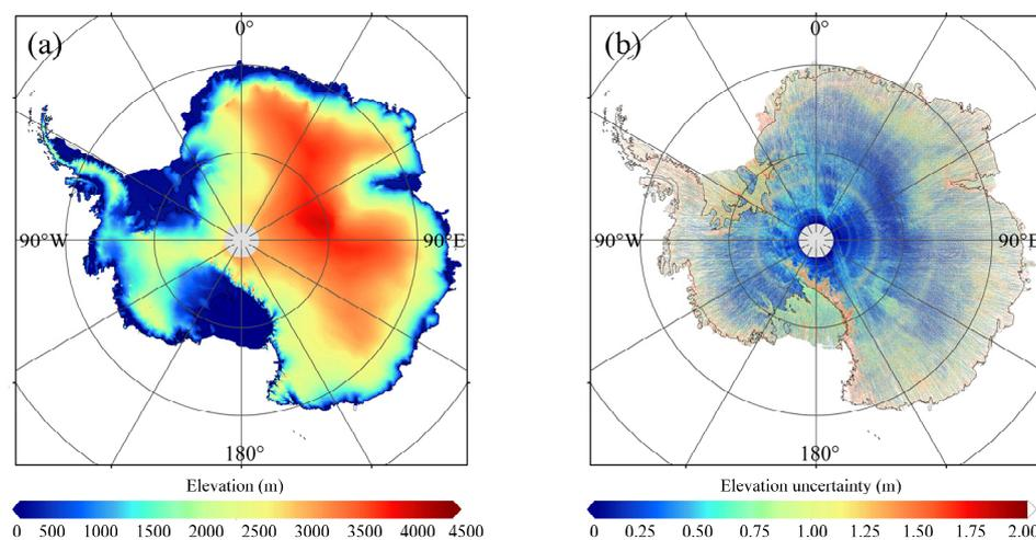
**Figure 4.** (a) A fine-scale DEM of Antarctica at a posting of 500 m derived from ICESat-2, which covers both the ice sheet and ice shelves with the southern limit of 88°S. (b) Map of the ICESat-2 DEM elevation uncertainty.
