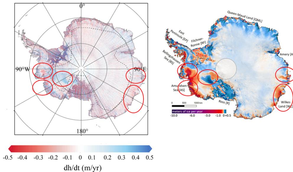
**Figure.** Map of elevation change rate in Antarctica derived from one year of ICESat-2 data in this study (left) and map of elevation change rate in Antarctica from 2003 to 2019 in Smith et al. (2019) (right).
