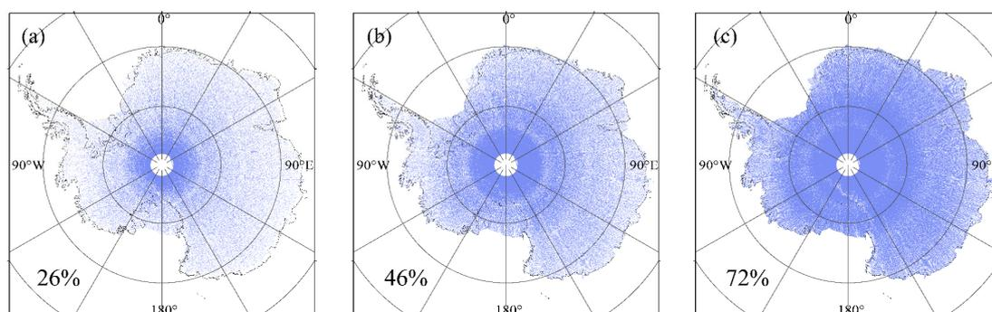
**Figure 2.** Map of the observed grid cells of DEMs at the spatial resolution of 250 m (a), 500 m (b) and 1 km (c). The observed grid cells are colored in blue, the overall coverage of each DEM in Antarctica is also presented beside.
