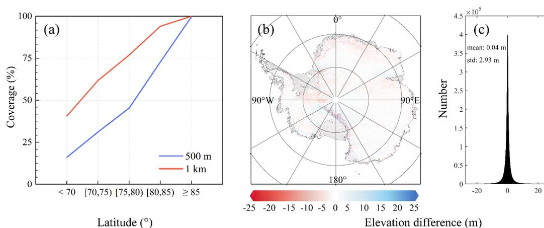
**Figure 3.** (a) Spatial coverages of observed grid cells in the five latitude ranges when two spatial resolutions, i.e., 500 m (blue) and 1 km (red), are applied. (b) Map of the elevation difference of DEMs at the resolutions of 1 km and 500 m. (c) Histograms of the elevation difference of DEMs at the resolutions of 1 km and 500 m, the average and standard deviation values are also presented.
