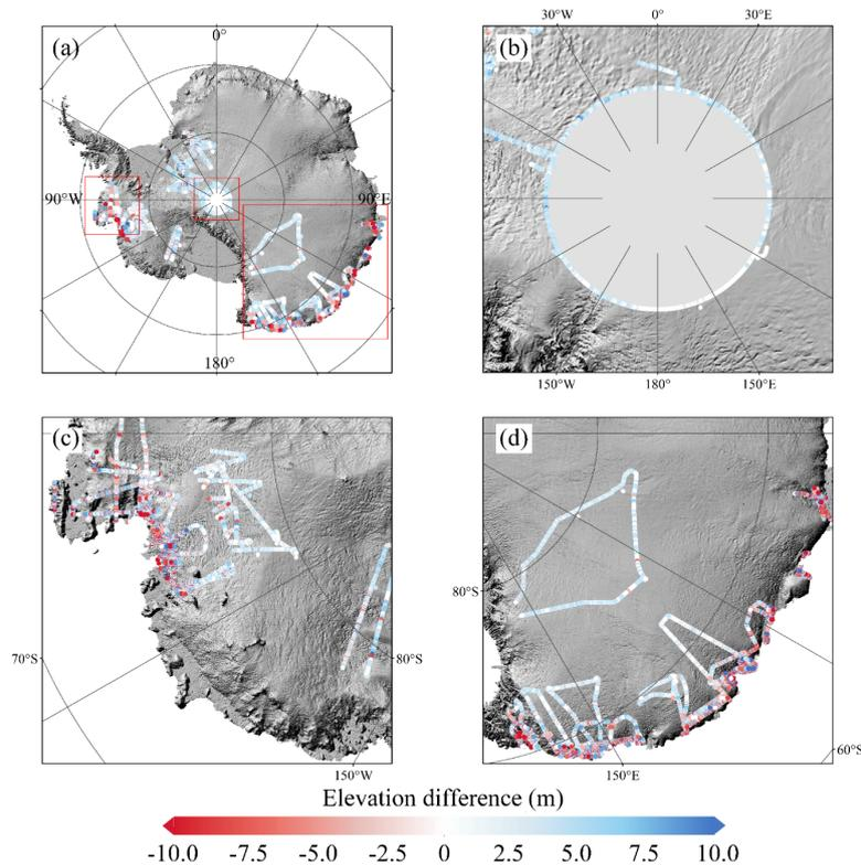
Figure 8. (a) Map of the difference between the ICESat-2 DEM and OIB airborne elevation measurements. Detailed maps of the ice sheet interior, Pine Island Glacier region and ice sheet margin in East Antarctica are shown in (b), (c) and (d), and their locations are also shown in (a) by red rectangular boxes. The background is the shaded relief map of Antarctica derived from the ICESat-2 DEM.
