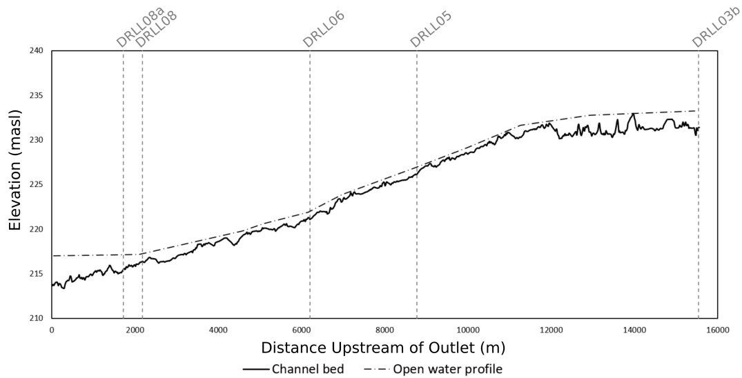
Figure 2. Channel bed profile of the Lower Dauphin River, with selected study locations, flow 86 \text{ m}^3/\text{s}
