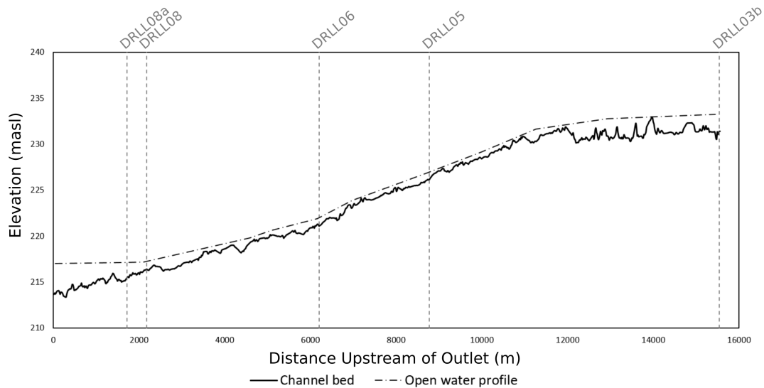
Figure 2. Channel bed profile of the Lower Dauphin River, with selected study locations, flow 86 \text{ m}^3/\text{s}
