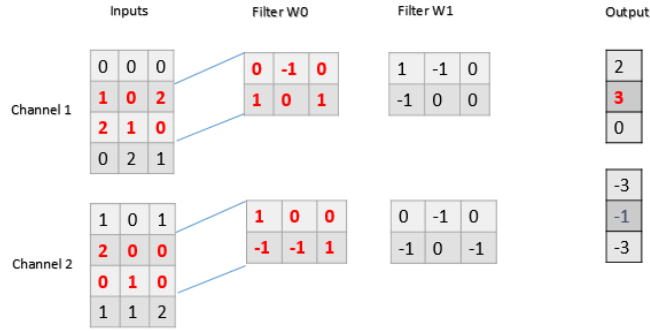
271 272 Figure 6. Structure of a convolution layer including two sets of filters.
