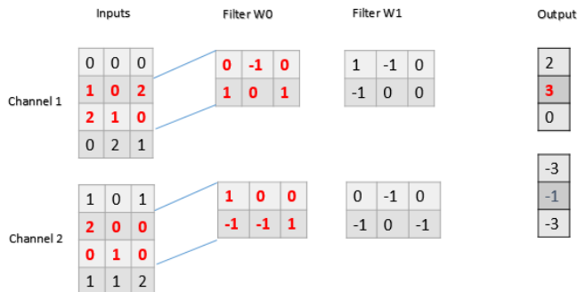
248 249 Figure 6. A convolution layer structure including two sets of filters.
