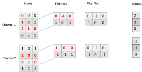
Figure-6. A Structure of a convolution layer structure including two sets of filters.
