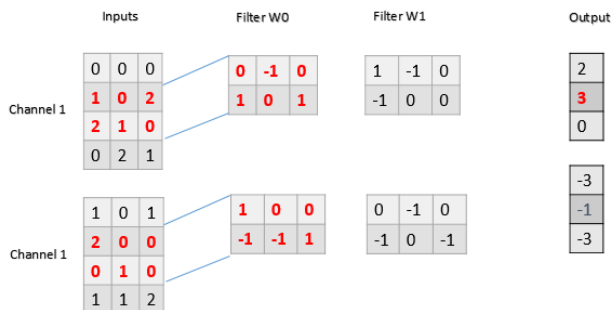
Figure 6. A convolution layer structure including two sets of filters.
