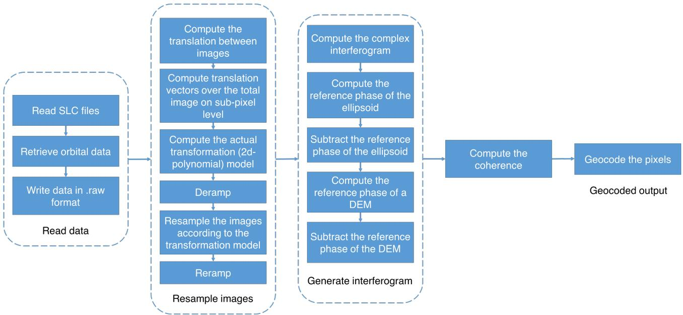
**Figure 2.** Delft Object-oriented Radar Interferometric Software (DORIS) processing flowchart from the software documentation available online at [http://doris.tudelft.nl/software/doris\\_v4.02.pdf](http://doris.tudelft.nl/software/doris_v4.02.pdf), customised based on Nikaein et al. (2021).
