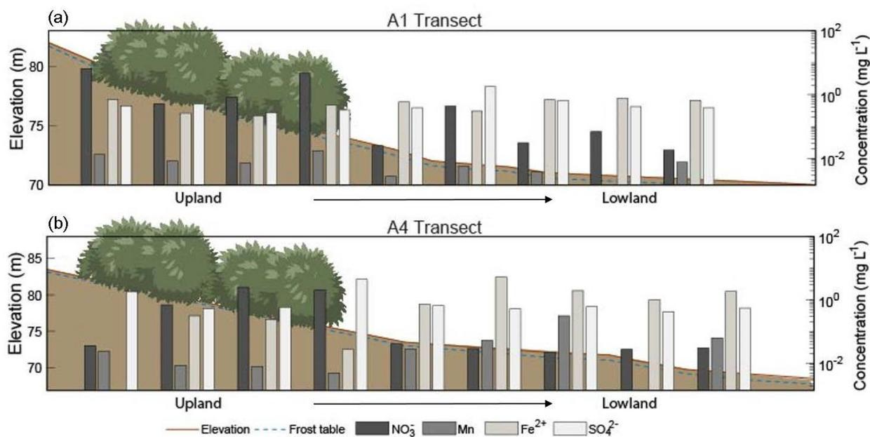
610 **Figure 4:** Elevation profiles and chemical concentrations along (a) A1 and (b) A4 transects, extending from the upland area to the lowland area during July (2018) sampling. Note that the elevation scale is different for A1 and A4 transects. Horizontal axis and shrubs not to scale. Depth to frozen soil or bedrock is depicted by the blue dashed line and shrubs indicate sample sites located within the alder shrubland. Redox
