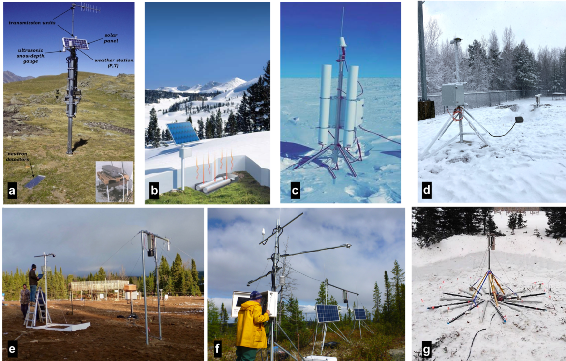
158 Figure 2. Photographs of sensors that were analyzed. a ) Cosmic Ray Neutron Probe (CRNP) from the EDF 159 French network (Nivomètre à Rayon Cosmic_NRC) at the Lac noir station in Ecrins-Pelvoux massif, France. 160 One can see the neutron probe buried in the ground (also shown in inset) and the mast, which carries 161 ancillary meteorological sensors. Credit: Delunel et al. (2014). b ) SnowFox CRNP set at ground level 162 beneath the snow cover. Similar to (a), the system requires measurements of atmospheric conditions. 163 Credit: Hydroinnova SnowFox manual. c ) Same sensor as in (b), but the Hydroinnova CRS-1000/B sensor is 164 placed above the snow, measuring ambient and upward neutron counts, with the latter being attenuated 165 by the snowpack. Crédit: Philip Marsh, Wilfrid Laurier University, Waterloo, ON, Canada; sensor in the 166 tundra at Trail Valley Creek, Changing Cold Regions Network http://ccrnetwork.ca . d ) GNSSr 167 installed at the Université de Sherbrooke SIRENE site. The antenna that was placed on the ground (beneath the snow) 168 was made visible at 3 m from the mast, on top of which a second antenna was affixed. Credits: Alain 169 Royer. e ) The FMCW-Radar (on the left) and the GMON (on the right) at the NEIGE-Forêt Montmorency 170 site. A metallic plate on the ground in the field-of-view of the radar substantially increases radar echoes. 171 In the background of photo (e), one can see the solid precipitation gauge, which is known as the Double 172 Fence Intercomparison Reference (DFIR). Credits: Alain Royer. f ) Meteorological and snow (GMON) 173 automatic station at the LeMoynes James-Bay, Québec, Canada site in a sub-arctic environment (Prince et 174 al., 2019). Credits: Alain Royer. g ) The GMON at the NEIGE-Forêt Montmorency site set up to boost 40 K 175 counts with pipes filled with potassium fertilizer. Credit: Sylvain Jutras.
