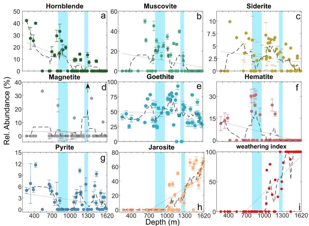
330 **Figure 6.** The variation of the major Fe-bearing minerals in TALDICE dust with depth. Dashed lines correspond to a 5-point moving average, solid grey lines to linear trends. In panel d, one sample-point is out of scale (black arrow, magnetite rel. ab. 70%). Panel i shows the weathering index, defined as the % ratio between jarosite concentration and the sum of jarosite, hornblende, muscovite and hematite.
