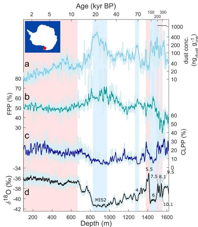
**Figure 1.** The mineral dust record of TALDICE. From the upper to the lower curve: (a) total dust concentration of insoluble particles (Baccolo et al., 2021); (b) FPP (fine particle percentage); (c) CLPP (coarse local particle percentage); (d)  $\delta^{18}\text{O}$  (Stenni et al., 2011). Light blue bands highlight glacial culminations (MIS 2-4-6-8), the red bands the Holocene and MIS 5.5, 7.5 and 9.5. In the upper-left corner the position of Talos Dome in Antarctica.
