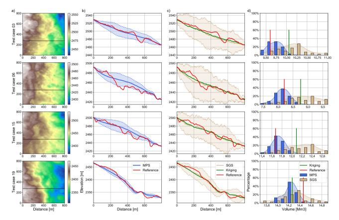
**Figure 6.** Synthetic test results. a) displays the reference DEM on a plan view, the black line showing the location of the cross-sections. b) presents the distribution of the cross-section simulated with the MPS method (parameter set 3). c) presents the distribution of the cross-section simulated with the SGS methods (parameter set 1). d) presents the different volume distribution of the methods against the reference one in red.
