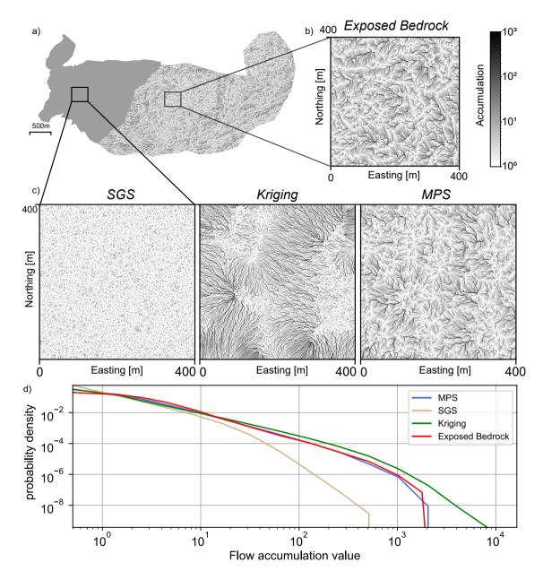
**Figure 9.** Flow accumulations calculated from the three methods and compared against the one computed in the exposed part of the bedrock used as reference, and the probability density of accumulation values. The SGS simulation under-estimates the length of the connected path, while kriging over-estimates overestimates it. The visual patterns and the flow accumulation distribution obtained with MPS are the closest to the exposed bedrock reference.
