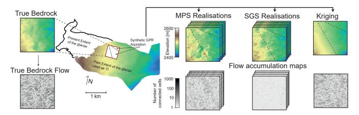
**Figure 4.** The approach used for the systematic tests. Test zones are extracted from the exposed glacier bedrock. GPR lines are also extracted from these zones and used to constrain the geostatistical simulations. It is then possible to compare the different sets with the actual topography. Flow accumulations maps are calculated from the simulated topography and from the reference extracted DEM for comparison.
