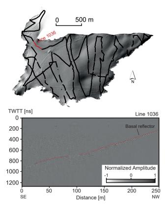
**Figure 2.** Acquisition lines from August 2018. The cumulative length is about 18km. Hill shade from the DEM derived from Drone images. The straight lines visible on the hill shade are ski lifts and transit tracks for snow groomers. A GPR line is displayed, with the basal reflector outlined.
