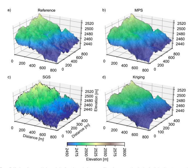
**Figure 5.** 3D view of topographic interpolation from the synthetic test case. The color correspond to the simulated elevation. a) presents the reference topography of the test case. b) a MPS simulation, c) a SGS simulation and d) a corresponding kriging estimate. The roughness is overestimated in with the SGS and underestimated with the kriging estimation. MPS simulation provide an acceptable compromise between the method and produce realistic structures.
