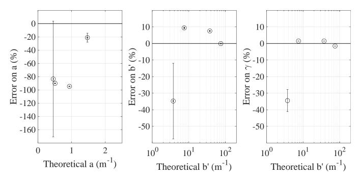
Figure 7: Validation of IOPs measurements using reference media. The reference media were 4 solutions of polystyrene microspheres in distilled water. Microspheres concentrations were chosen for the theoretical a and b' ranges to cover sea ice typical values. Detecting fibres 1 and 7 were taken out for optimized results.
