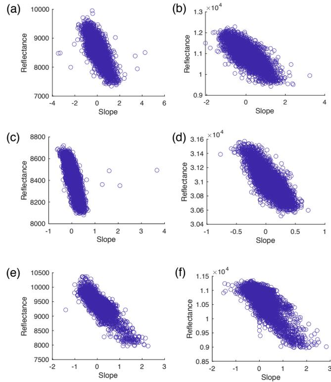
**Figure A1.** Plots of slope vs. Landsat-8 red band reflectance for areas outside of the lake and buffer zone for each of the Landsat-8 images analyzed for the photoclinometry portion of this study. The plots are laid out as follows: (a) Lake 2 Before, (b) Lake 2 After, (c) Lake 5 Before, (d) Lake 5 after, (e) Lake 6 Before, and (f) Lake 6 After. ~~Images are the same as those in A2-~~
