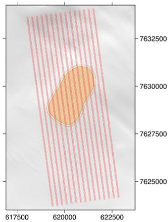
**Figure A2.** Lake 6 transects for photogrammetry calculations for image on 28 Oct 2016 prior to drainage (red), lake extent (orange) and buffer (yellow). For description of how these features are used in the photogrammetry calculations, see Methods.-
