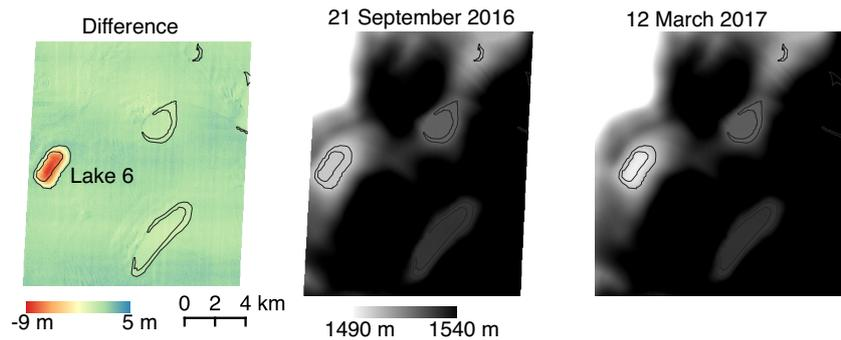
**Figure 8.** Elevation difference results of the photogrammetry-ArcticDEM analysis ~~beside the before and after images (Landsat-8 Red Band, B4) to illustrate confirm~~ the visible physical changes to observed in the lake lid before Sentinel-1 imagery and after drainage. The first column of images shows the collapse vertical distance of each pixel. It is the result of interpolating and differencing the pre- and post-drainage topography as mapped out by photogrammetry analyses.
