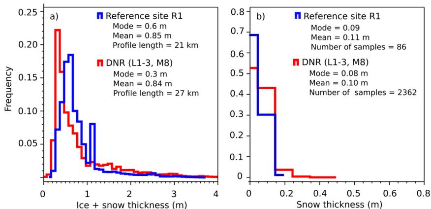
**Figure 6:** Total (ice plus snow, a) and snow (b) thickness distribution of the floes located inside the DNR (L1-3, M8, red line), and at R1 (blue line, see Fig. 3a for positions). Ice thickness measurements were made with a ground-based electromagnetic (GEM) instrument pulled across the ice on a sledge. Snow thickness measurements were made with a Magna Probe.
