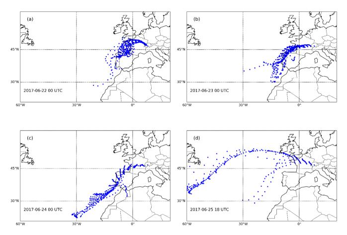
Figure 4: 5-day air mass backward trajectories starting from the Jungfraujoch site at 00 UTC on 22<sup>nd</sup> to 24<sup>th</sup> June 2017. For 25<sup>th</sup> June starting time is 18 UTC.
