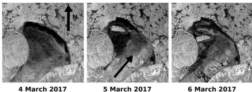
Figure 17. Sequential Sentinel-1 images showing the breakup and drift of an ice piece that was labelled floe #39 in this study. This modulated 515 the ice arch. The arrow indicates the dominant wind direction between the acquisition times of the images for 4 and 5 March.
