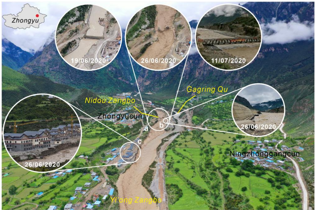
Figure 12.3. Examples of GLOF damage to downstream infrastructure and buildings at the confluence of Nidou Zangbo and Gagrang Qu. Background aerial photo by H. Li taken on 26 June 2020. (a) Comparison of the bridge connecting Zhongyucun and Ningzhonggangcun before, during (photos: H. Li) and after the GLOF (rebuilt, photo: K. Ma). (b) Destroyed roads (photo: H. Li). (c) Affected buildings at risk (photo: H. Li).
