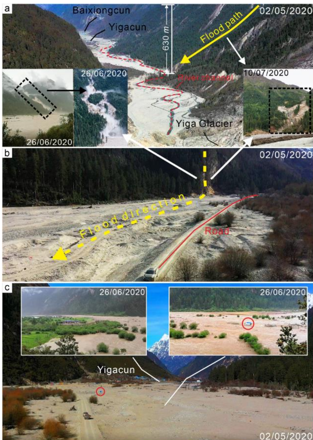
Figure 112. The situations in the valley and river channel below Jinwuco before, during, and after the GLOF. (a) Photo taken from Yiga Glacier looking to Yigacun. Insets showing the situations in the valley during and after the GLOF (photos: Q. Quying and Y. Quzhen). (b) The river channel and road before the GLOF taken from Yigacun looking upstream. The yellow dashed line is the flood flow direction. (c) A view taken from upstream looking to Yigacun. Insets showing the situations in the river channel during the GLOF (photos: Q. Quying). Aerial photos from 2 May 2020 were taken by K. Liang.
