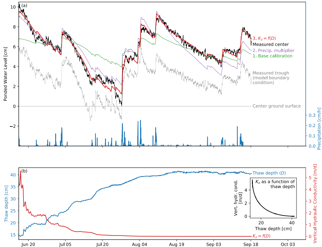
Figure 11 a) Progression of center water-level calibration. The (1) base calibration, (2) calibration with a precipitation multiplier, and (3) calibration with vertical hydraulic conductivity as a function of thaw depth ( K_z = f(D) ). The measured polygon-center and trough water levels are plotted for reference. Precipitation is plotted on the right y-axis. (b) Measured thaw depth and calibrated vertical hydraulic conductivity as a function of thaw depth.
