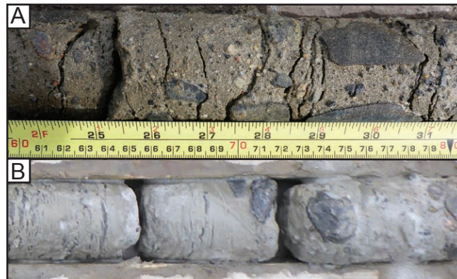
Figure B4. Evidence of permafrost in previously thawed till. (A) Thin lenses of segregated ice at 3.3–3.5 m in NGO-DD15-1007 indicate refreezing of thawed till and illustrate the different appearance when compared to the cryostructure in Fig. B3. (B) The contact between the well sorted silt/sand and coarser material at 3.7–4.1 m in NGO-DD15-2012.
