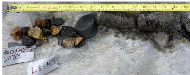
Figure 7. Heating of the drill barrel, likely due to cutting through the rock near the middle of this section, caused complete melt of ground ice in the left part of the core shown. Here, gravel was recovered but fines were likely washed out with melt water and drilling fluids. The right side of the core is partially thawed and ice rich. This recovered section of less than 0.5 m represents 1.3 m in borehole NGO-DD15-2033.
