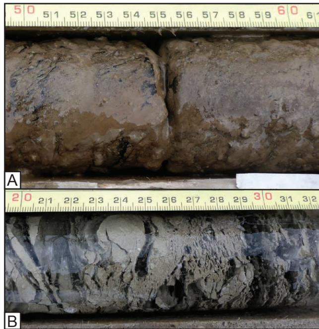
**Figure B1.** Drill core recovered from borehole NGO-DD15-1010 in the Valley. (A) shows core from 1.6 m depth with 46 % excess ice and 1.3 % organic matter. (B) is about 3.5 m depth with 60 % excess ice and 1.5 % organic matter. Scale bars are in cm.
