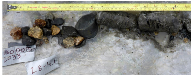
Figure 7. Heating of the drill barrel, likely due to cutting through the rock near the middle of this section, caused complete melt of ground ice in the left part of the core shown. Here, gravel was recovered but fines were likely washed out with melt water and drilling fluids. The right side of the core is partially thawed and ice rich. This recovered section of less than 0.5 m represents 1.3 m in borehole NGO-DD15-2033.
