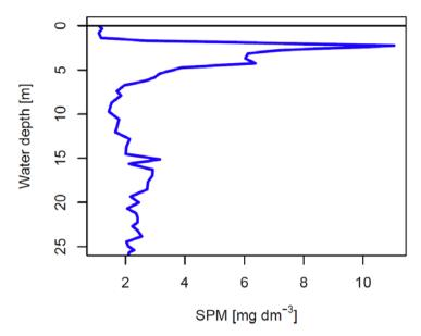
1088 Fig 3. Turbidity profile of the SG station converted to suspended particles.
