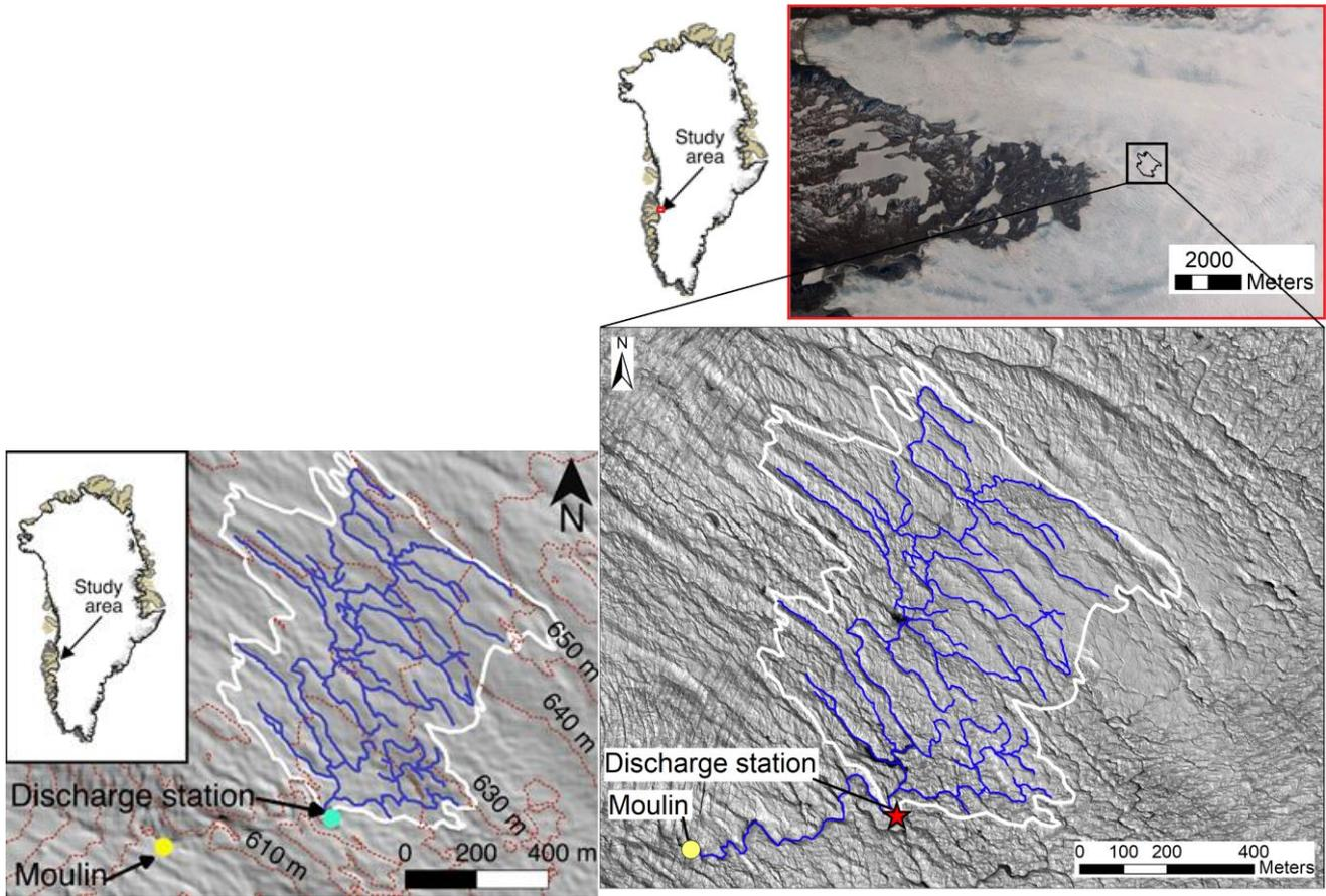
Figure 1: Map of study site showing the supraglacial catchment boundary (white), streams of order 1, 2, and 3 (blue), and locations of the discharge station and terminal the moulin. ~~Red contour lines are derived using a 10-m Arctic DEM from Polar Geospatial Center (PGC). Hillshading is generated from a PGC 2m DEM.~~
