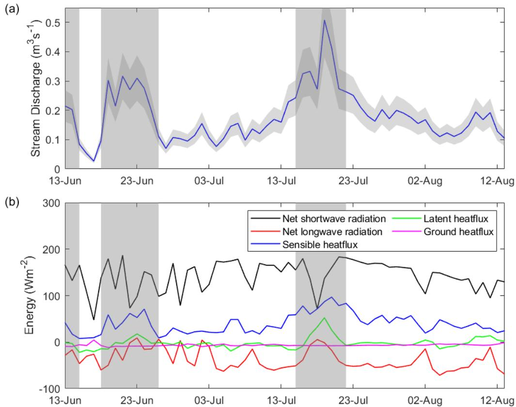
Figure 6:(a) Daily discharge measured by averaging the hourly discharge from Fig. 5a. Uncertainty of daily mean discharge generated by averaging hourly discharge,  $X_{dm}$ , is shown in the grey shaded area (see Appendix A for uncertainty calculations), (b) surface energy components, net shortwave radiation (black), net longwave radiation (red), sensible heat flux (blue), latent heat flux (green), and ground heat flux (magenta). Large melt episodes are shown in grey shaded regions.
