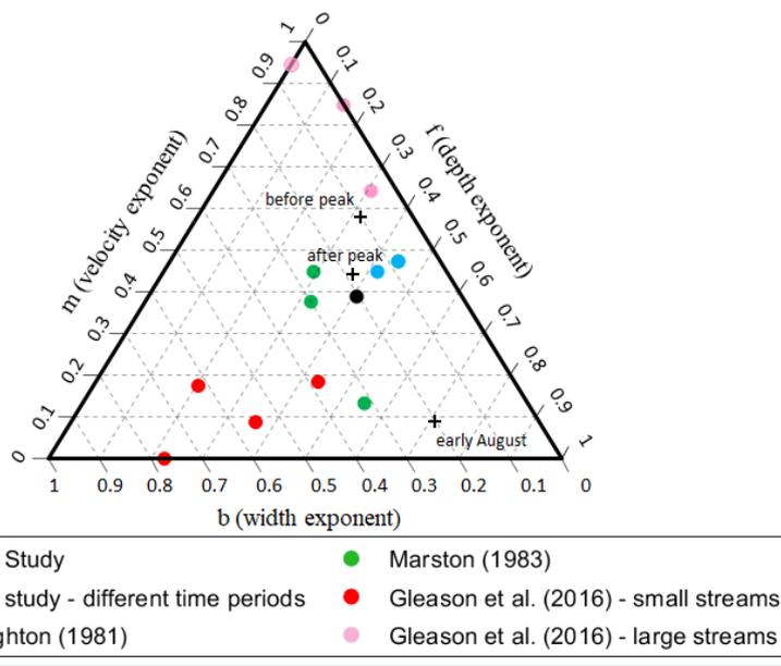
**Figure 110:** Ternary diagram comparing  $m$ ,  $f$ , and  $b$  parameters from this study (in black; whole season in solid dot, different time periods in '+' with before peak - 17 June–20 July, after peak - 26–27 July, and early August - 4 August) with previous work by Knighton (1981) in blue, Marston (1983) in green, and Gleason et al. (2016) large streams in pink and small streams in red. Where  $m+f+b$  exceeded unity, parameters were adjusted to unity.
