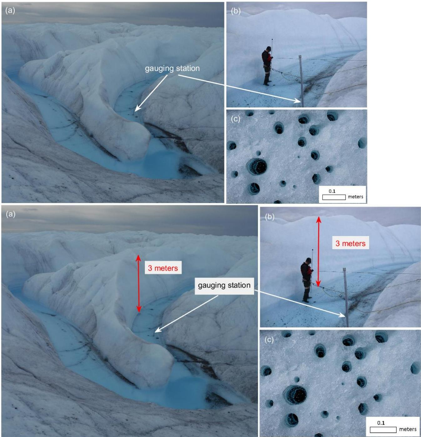
Figure 2: (a) ~~The main stem of the s~~Supraglacial stream main stem, and ~~location of the~~ gauging station location. (b) Close up photo of the stream cross-section, and the gauging station during discharge measurement. (c) Cryoconite holes on the bare ice surface vary from 0.02–0.08 m in diameter and 0.1–0.3 m in depth (in this figure). These holes are partially water filled and contain cryoconite (biological matter), dust, and sediment at the bottom.
