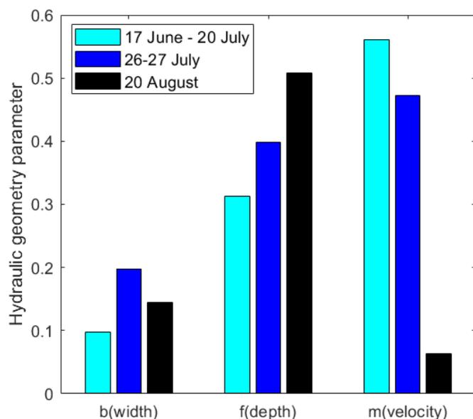
**Figure 10: Hydraulic geometry parameters calculated for three different times, 1) bulk of melt season before peak (melt episode in July), 2) after the peak (melt episode in July), but before increase in peak timing, 3) after the peak (melt episode in July), and after increase in peak timing (in early August).**
