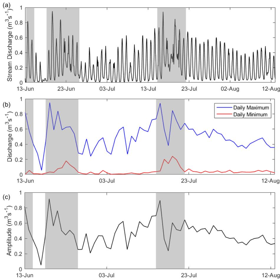
310 **Figure 5: (a) Hourly stream discharge generated using the rating curve (Fig. 4) over 62 days of the melting season. (b) Daily maximum (in blue) and daily minimum (in red) discharge, calculated from the hourly discharge. (c) Amplitude (daily maximum minus daily minimum) of the stream discharge. Three large melt episodes are shown in grey shaded regions.**
