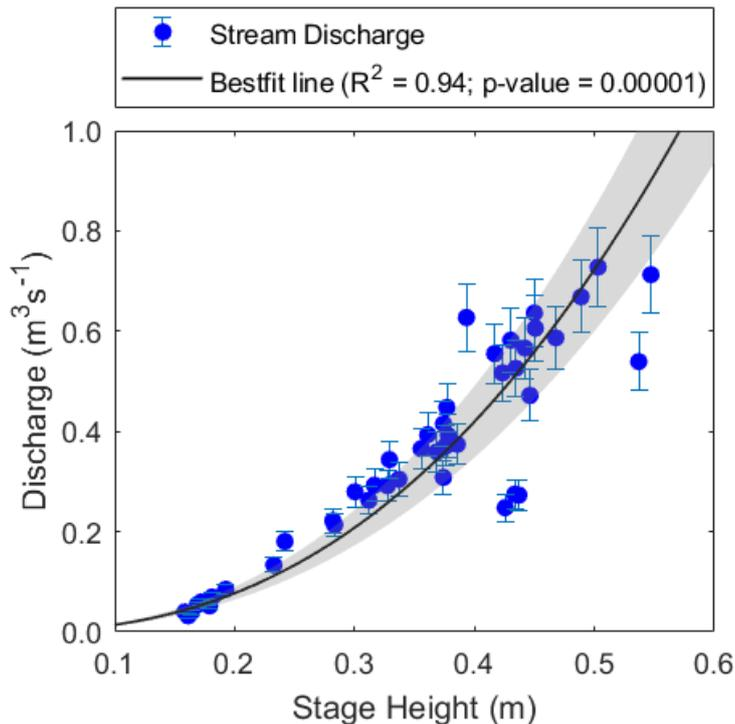
215 **Figure 4: Rating curve (black line) determined from the best fit of power law (Eq. 1) to observations of stage and discharge (blue dots). Error bars show measurement error uncertainty ( $U_{me}$ ). Rating curve uncertainty ( $U_{RC}$ ) is shown in the grey shaded area (see Appendix A for uncertainty calculations).**
