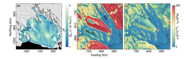
Figure 2. Panel (a) shows the inverse rate factor  $\bar{B}_{inv}$  in the floating part of the model domain. The value of uniform  $\bar{B}_u$  is shown in the colourbar of panel (a). Panels (b) and (c) focus on MacIS and BIS, showing the friction coefficient  $\alpha$  and corresponding basal drag  $\tau_b = -\alpha^2 N \mathbf{u}_b$ . The grounding line is the observed position from Bindschadler et al. (2011).
