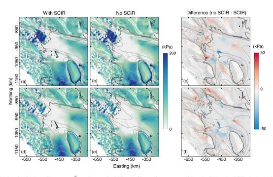
Figure 7. The longitudinal tensile stress  $+\bar{R}_{ll}$  acting on the RIS and tributary ice streams with and without the SCIR. In (a-c), the simulation is initialised with  $\bar{B}_{inv}$ . In (d-f), the simulation is initialised with  $\bar{B}_u$ . In (a) and (b), the unusually high  $+\bar{R}_{ll}$  values at the outlet of MacIS and BIS are due to relatively high  $\bar{B}_{inv}$  values inferred during model initialisation.
