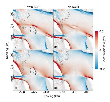
Figure 12. Model shear strain rates near the SCIR for (a) and (b) spatially variable ice properties ( $\bar{B}_{inv}$  model) versus (c) and (d) uniform ice properties ( $\bar{B}_u$  model). Grounding-line positions are from the appropriate  $\bar{B}_{inv}$  or  $\bar{B}_u$  reference and perturbed models.
