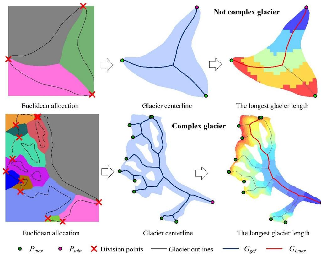
**Figure 6: The schematic of extracting glacier centerlines and the longest glacier centerline.**
