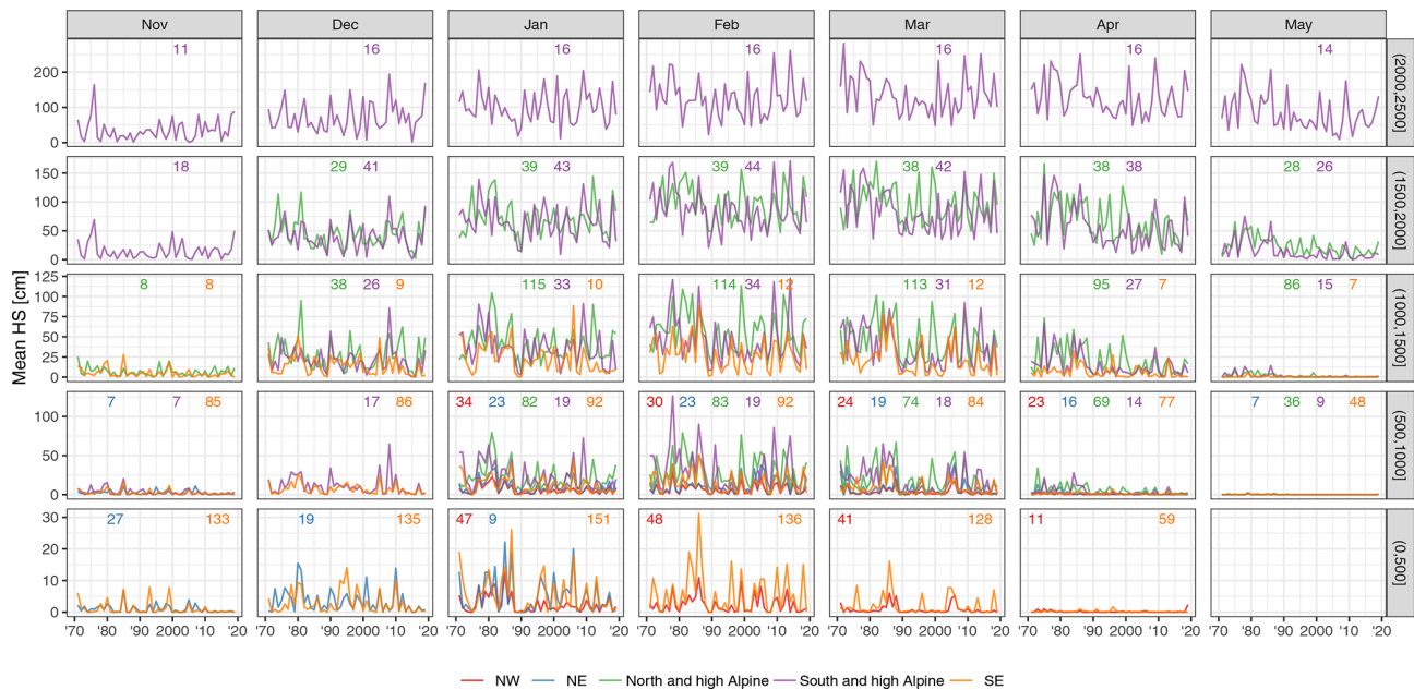
Figure 8. Time series of mean monthly snow depth averaged by 500 m elevation bands. The rows indicate elevation band and the columns the months. The small numbers at the top of each panel denote the number of stations included in the average. Lines are only shown if more than five stations were available. Time series of all single stations are available in the repository (Matiu et al., 2020).
