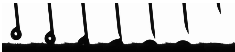
165 Fig. 2. Process of the contact angle measurement between the aqueous ethylene glycol solution and black 166 soil at -10°C.
