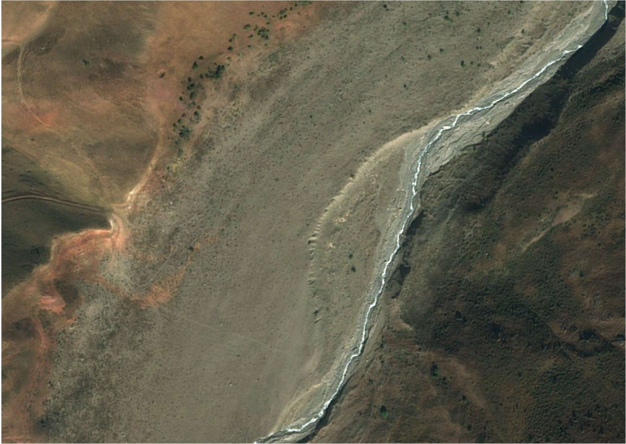
Fig. S3: Later deposit area of the Rasht 2019 detachment showing features of a potential earlier ice-rock avalanche (streamlined features to the middle and lower part; rough chaotic microtopography to the upper right). (© GoogleEarth, Maxar).
