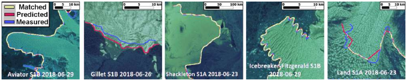
Figure 12. B-VS Validation Output Results: Similar to Z-NN, B-NN uses a high resolution input (768×768) relative to CALFIN-NN (224×224), which skews the mean pixel distance comparison in CALFIN-NN’s favor. See Fig. S11-S12 for full outputs.
