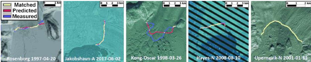
Figure 9. CALFIN-VS Validation Output Results: Yellow represents human (green) and machine (red) agreement on the front location. Note that the drop in mean pixel distance despite the increase in mean meter distance (and vice versa) comes from L7SCE images being reprocessed at lower sizes due to detection failures (see Fig. 6c), and pixel error bias being inversely related to input size (see Sect. 4.1).
