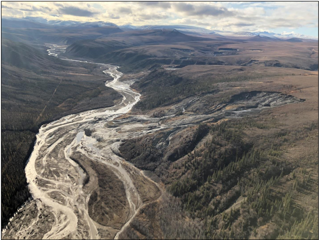
Figure S2. Willow River main stem view looking southwest. Photograph shows small shallow slides in foreground, and large deep-seated translational failures which have evolved into retrogressive thaw slumps. Slide materials have runout onto the braided floodplain. Numerous retrogressive thaw slumps are visible in background on slopes of incised tributary streams.
