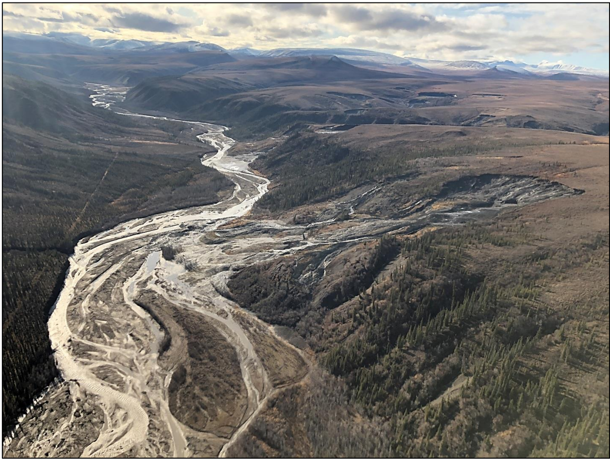
285 Figure S3. Willow River main stem view looking southwest. Photograph shows small shallow slides in foreground, and large deep-seated translational failures which have evolved into retrogressive thaw slumps. Slide materials have runout onto the braided floodplain. Numerous retrogressive thaw slumps are visible in background on slopes of incised tributary streams. Photograph is upstream view towards inset (b) on Figure 6.
