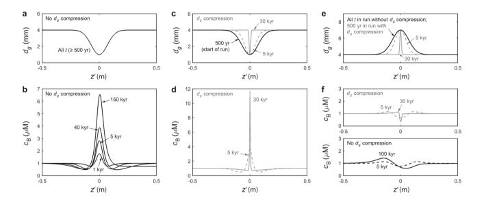
**Figure 12:** Four modified GRIP control runs, demonstrating how fluctuations in the mean grain size  $d_g$  (a, c, e) at decimetre scale cause signals to form on the bulk concentration  $c_B$  (b, d, f). All runs begin at t = 500 yr with  $c_B \equiv 1 \mu M$  without an initial impurity signal. Evolution
