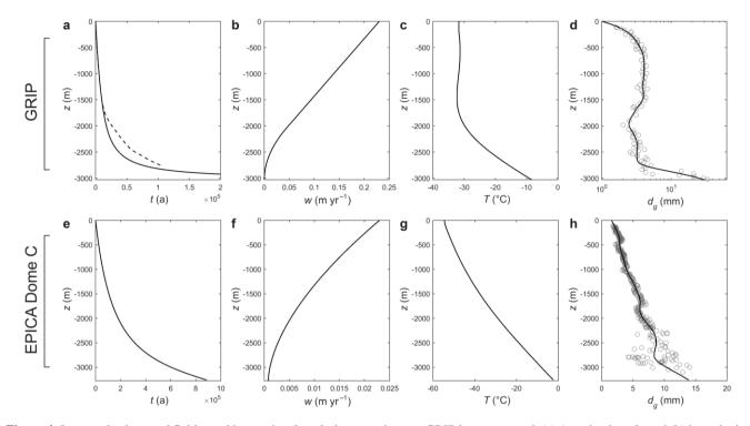
Figure 4: Ice-core background fields used in our signal evolution experiments. GRIP ice core: a to d. (a) Age-depth scale and (b) ice velocity from a Dansgaard-Johnsen model. Dashed line in (a) shows the GICC05 modelext time scale (Seierstad et al., 2014; Rasmussen et al., 2014).
