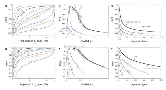
**Figure 8:** Changing morphometry of the signal peak – its amplitude, full width at half maximum (FWHM), age span – in the EPICA ice core for different model parameters, plotted against depth (a–c) and age of the ice (d–f). Black curves plot the control run of Fig. 6a, and orange curves the  $\gamma = 0$  run of Fig. 6d. Grey and blue curves document the same sensitivity tests as conducted for the GRIP core (see Fig. 7
