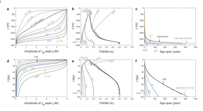
**Figure 7:** Changing morphometry of the signal peak – its amplitude, full width at half maximum (FWHM), age span – in the GRIP ice core for different model parameters, plotted against depth (a–c) and age of the ice (d–f). Black curves plot the control run of Fig. 5a, and orange curves the  $\gamma = 0$  run of Fig. 5d. Grey curves plot the results of altering the width parameter  $\Delta$  of the doped peak from 0.08 (control) to four
