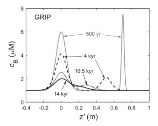
**Figure 10:** Snapshots (at four times) of the evolution of two neighbouring peaks in a GRIP run that uses the control parameters of the run in Fig. 5a. Diffusional spreading causes the peaks to merge as they approach each other under vertical compression. See Movie S3 for the full simulation.
