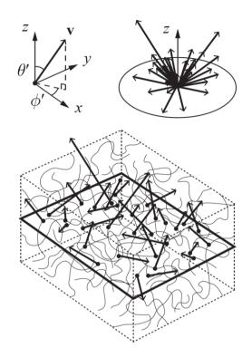
**Figure B1:** Velocities **v** of different vein segments crossing a plane (outlined by bold rectangle), and their distribution in spherical coordinates (upper right). Only crossings in one direction are shown. In Appendix B, a statistical theory is used to calculate the net transport of porosity and vein impurity resulting from this motion.
