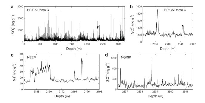
**Figure 1**: High-resolution records of dissolved ionic impurities in ice cores from Antarctica and Greenland, illustrating the occurrence and expressions of high peaks and signals at decimetre or shorter scale in deep ice. Vertical axes plot the total impurity concentration in bulk ice (this differs from our model variable  $c_B$ , which refers only to impurities in the water-vein network); 1 ng g<sup>-1</sup> is equivalent to 1 ppb or 1  $\mu$ g
