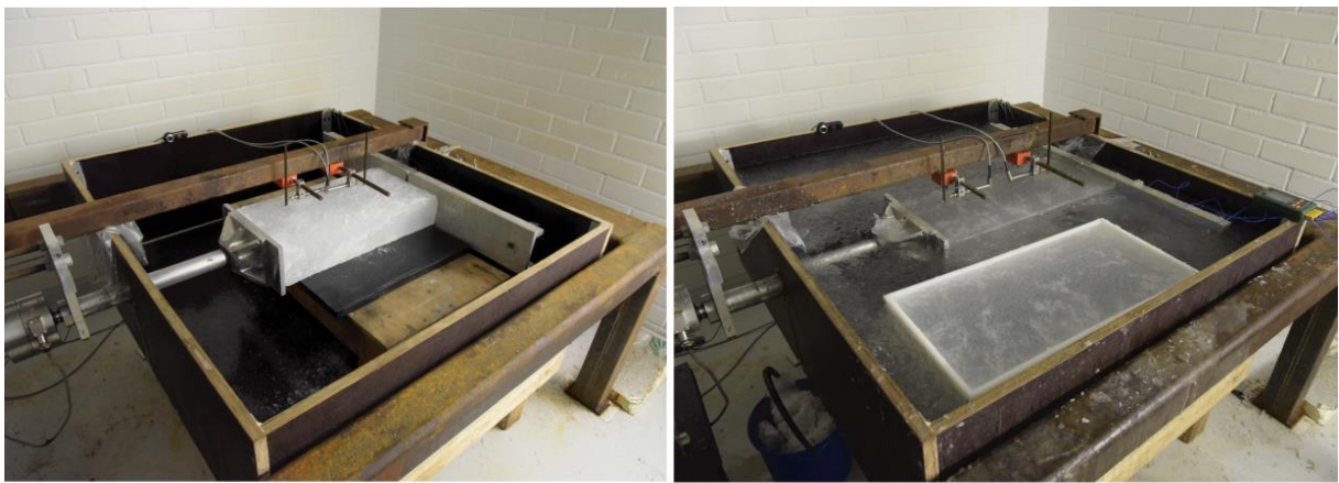
Figure 2. Equipment used in the (a) dry and (b) floating ice experiments. One of the plastic molds used when growing ice is shown in (b). The thin ice cover of the basin, seen in (b), was broken before performing the experiments.
