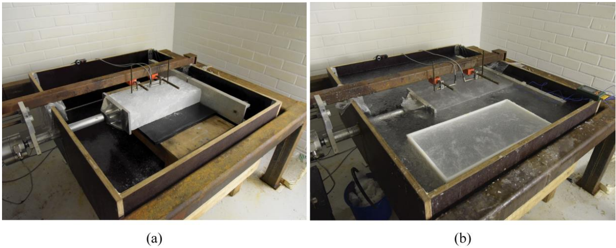
Figure 2. Equipment used in the (a) dry and (b) floating ice experiments. One of the plastic molds used when growing ice is shown in (b). The thin ice cover of the basin, seen in (b), was broken before performing the experiments.
