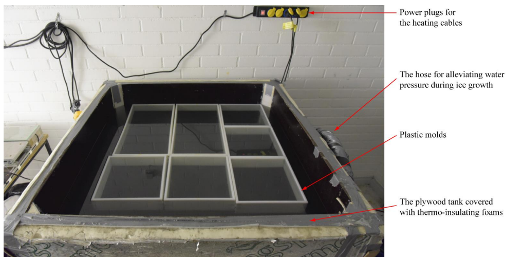
Figure 1. The tank made of plywood for growing ice specimens.
