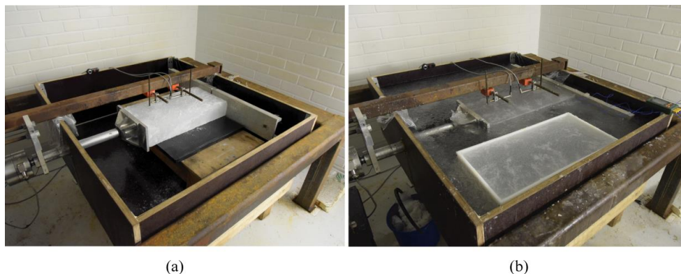
Figure 2. Equipment used in the (a) dry and (b) wet experiments. One of the plastic molds used when growing ice is shown in (b). The thin ice cover of the basin, seen in (b), was broken before performing the experiments.
