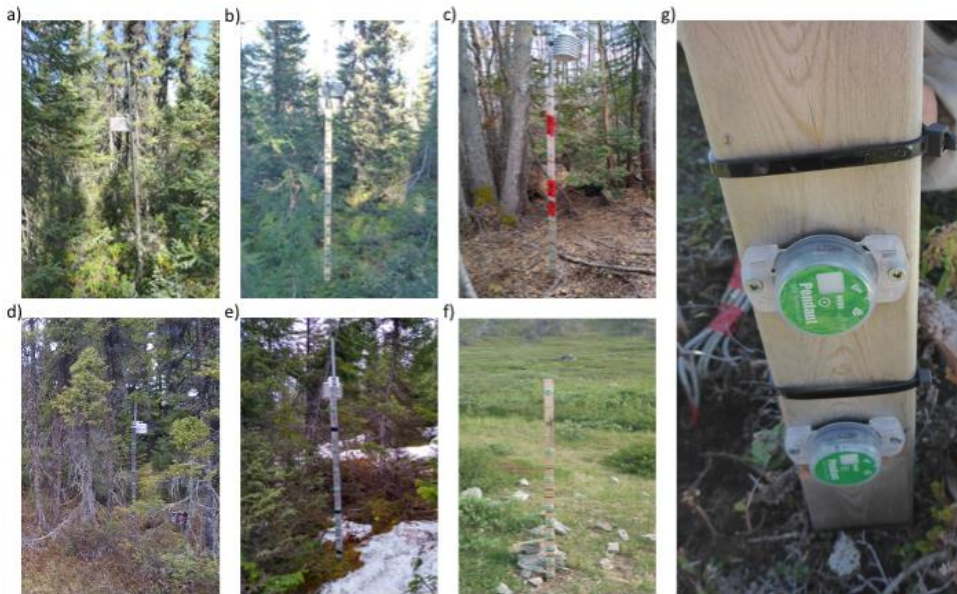
125 Figure 3: Field photos of all SCLT measurement sites for 2018-2019 and (g) a close up of logger installation onto stake. These include: (a) Amet11, (b) Amet12, (c) Amet17, (d) Amet28, (e) Amet29, and (f) BaseSnow.
