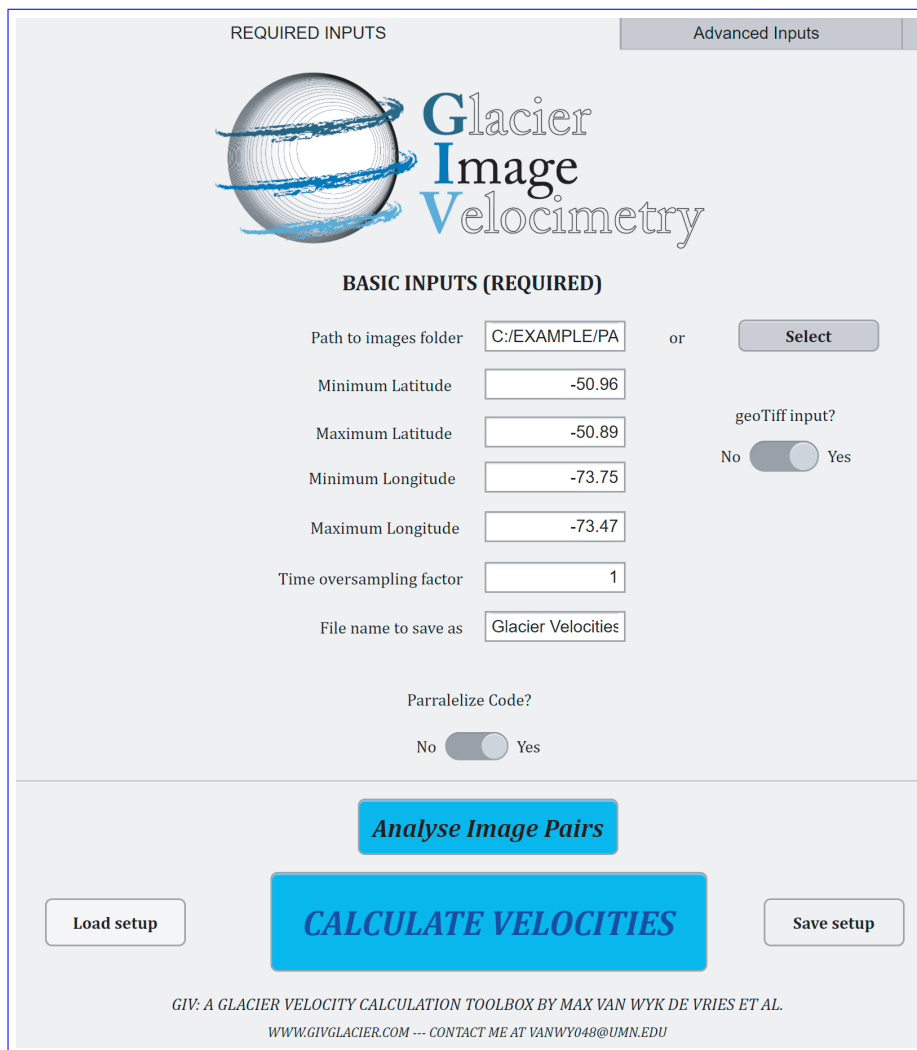
Figure 11. Main graphical user interface for GIV, showing the main input fields. This interface may either be run through MATLAB or as an independent desktop app with no licensing requirements.
