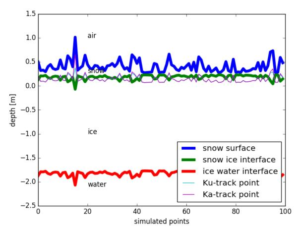
The figure is showing the air/snow, snow/ice and ice/water interfaces together with the simulated Ka- and Ku-band track points for the first 100 RRDP points.
