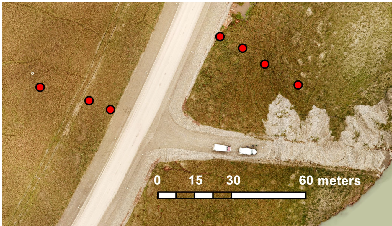
Figure A1: Transect of iButton soil temperature loggers across the Dalton highway at our site close to Deadhorse (70.099°N, 148.511°W). Red dots indicate the position of ibutton sensors, the bright grey element shows the gravel road surface, the adjacent darker grey elements show the road shoulders. To the right a side road leading to the adjacent Sagavanirktok River (lower right) is seen (drone photo Soraya Kaiser).
