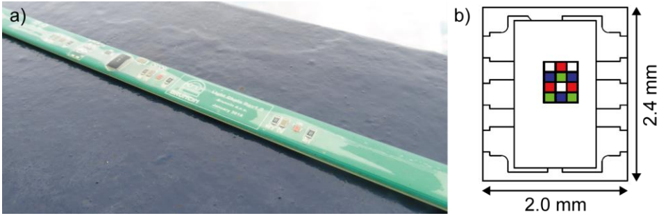
Figure 1: a) a segment of the chain prototype during the calibration procedure. The optical sensors are visible as red-colored components on the circuit board. The black addressing chip controlling the sensors of a particular chain section can be seen in the middle of the picture. b) Sketch of the arrangement of the different spectral channels on the 3x4 photodiode array of the sensor.
