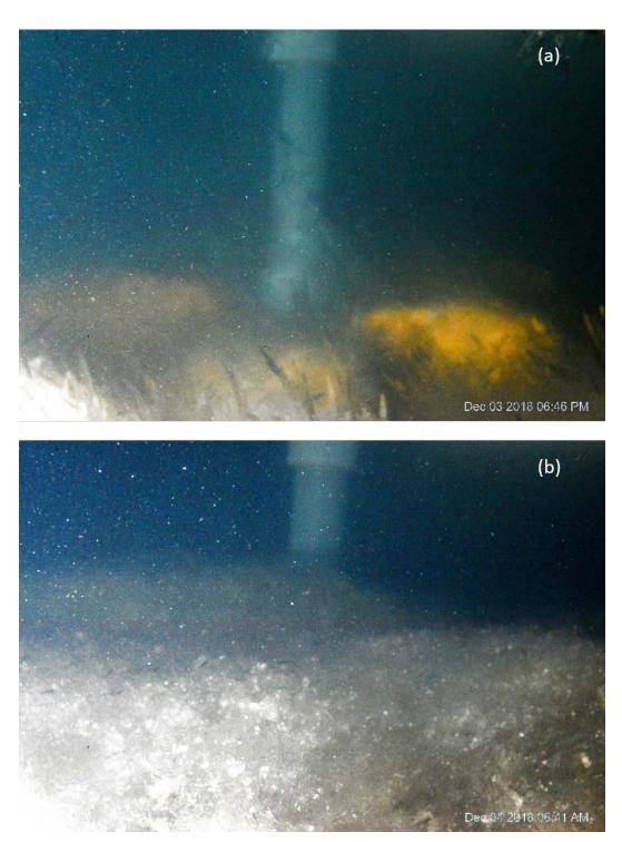
Figure 3: Sample processed images from an anchor ice event on Dec. 3&4, 2018 (Event C) showing: (a) individual crystals growing off the substrate, and (b) anchor ice accumulation over the substrate.
