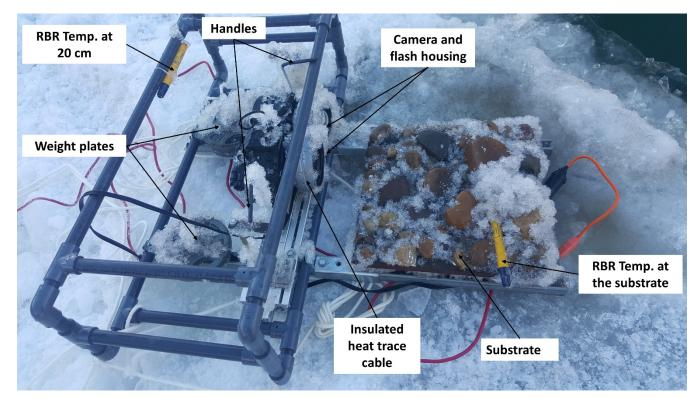
Figure 2: Anchor ice imaging system and artificial substrate after its retrieval from the river on Nov. 12<sup>th</sup>, 2018.
