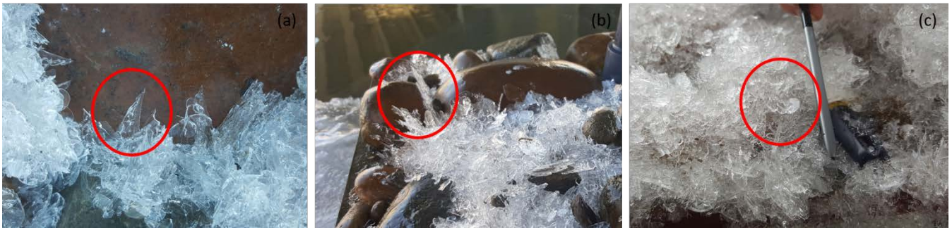
Figure 10: Observed anchor ice crystal types (highlighted with red circles) from the 2018 freeze-up season showing (a) curved needle crystals, (b) platelet crystals, and (c) disk crystals.
