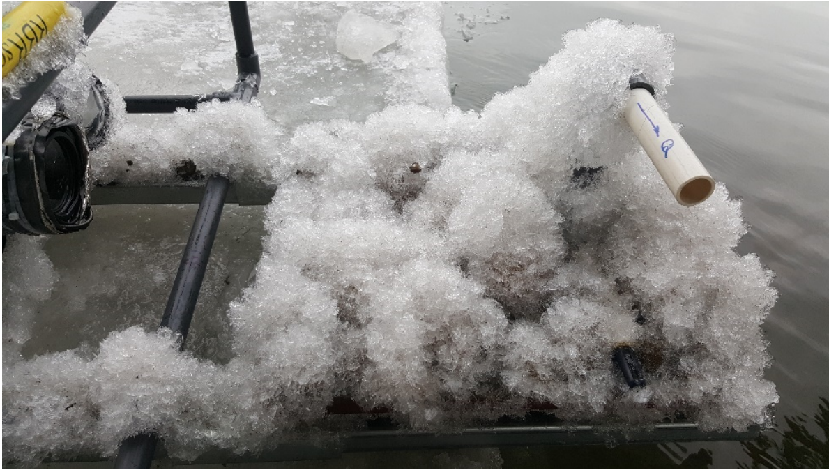
Figure 9: Anchor ice formation on the artificial substrate after the instrument's retrieval on 12-Nov-2018.
