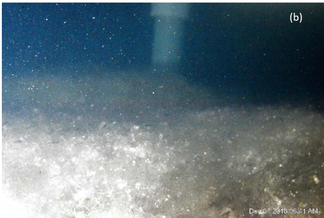
Figure 3: Sample processed images from an anchor ice event on Dec. 3&4, 2018 (Event C) showing: (a) individual crystals growing off the substrate, and (b) anchor ice accumulation over the substrate.
