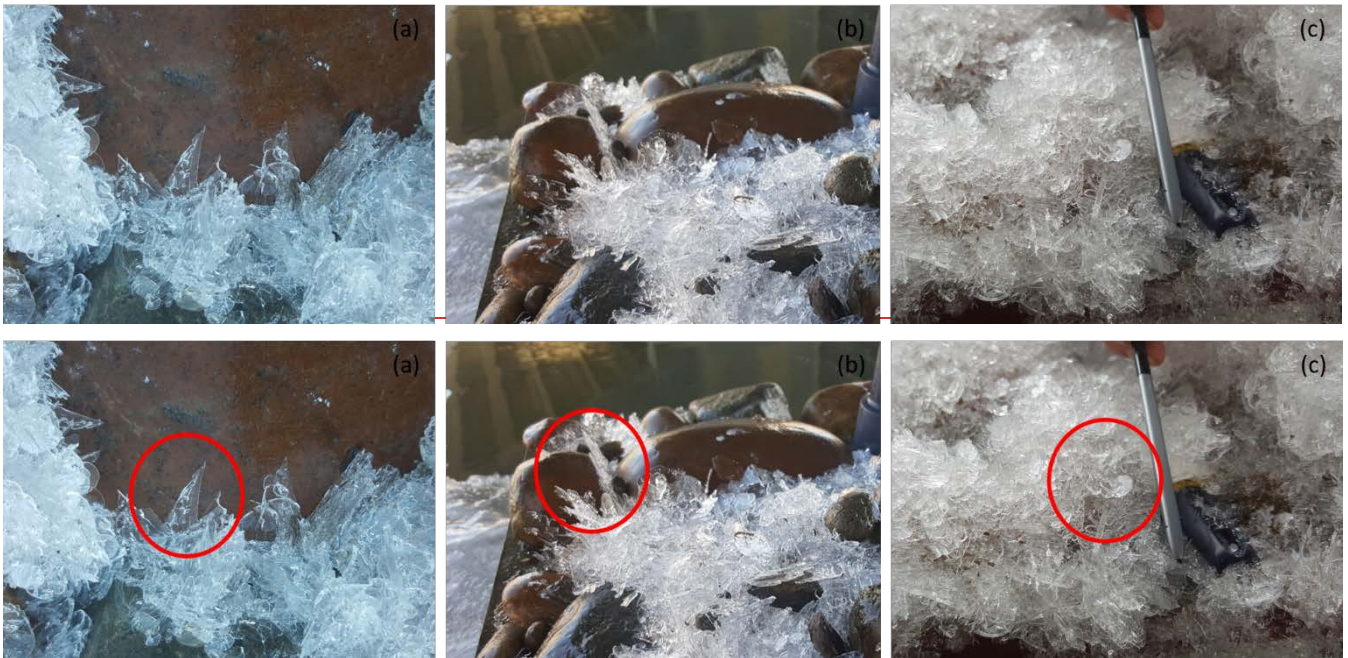
Figure 9: Anchor ice formation on the artificial substrate after the instrument's retrieval on 12-Nov-2018.
