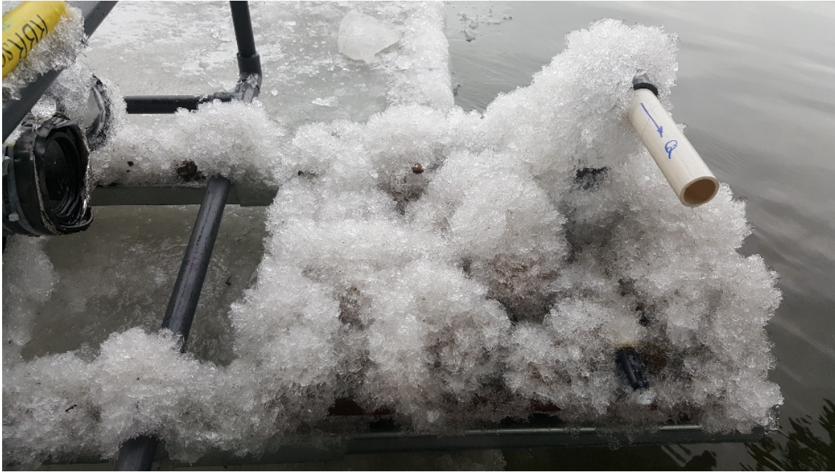
Figure 9: Anchor ice formation on the artificial substrate after the instrument's retrieval on 12-Nov-2018.
