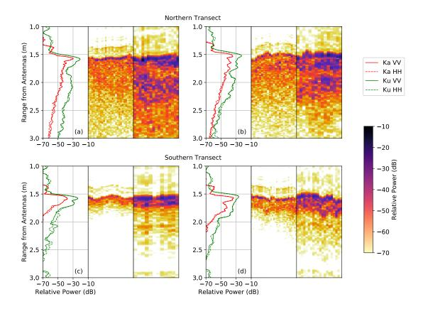
Figure 8. Average VV- and HH-polarized signal power as a function of range at Ku- and Ka-band for specific locations along the northern (a,b) and southern (c,d) transects as shown in Figure 7. The difference in the average spectrum between (a,b) and (c,d) is that they are from different locations along the transect and highlight the influence of multiple scattering in the snow and a return from what could be the snow/ice interface at Ku-band.
