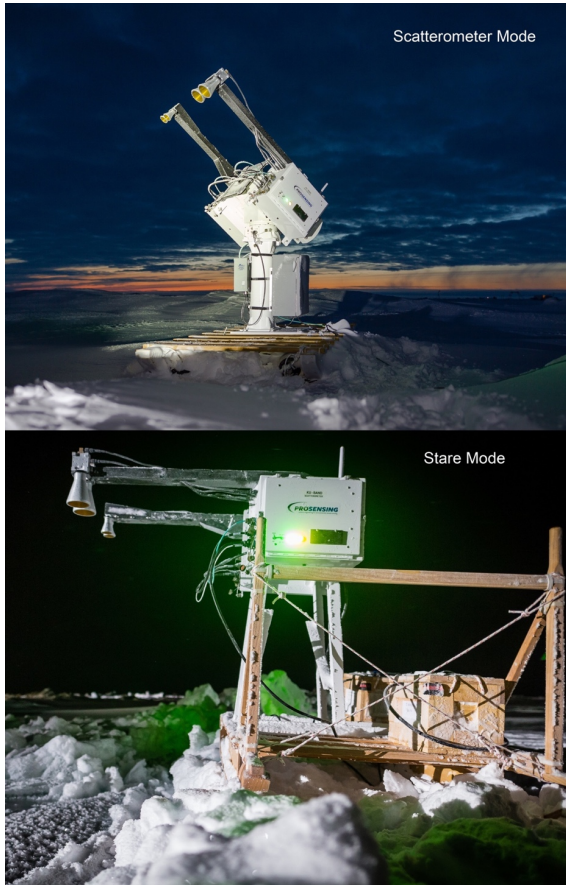
Figure 1. Configuration of KuKa radar in scatterometer “ scan ” (top) and altimeter “ stare ” (bottom) modes. Photo Credit: Stefan Hendricks.
