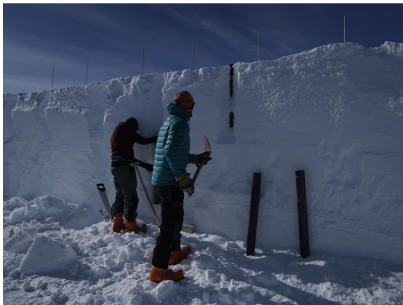
5 Figure 3: Sampling procedure in the OIR trench. The first carbon fiber liner is pushed into the snow after excavation of the trench. The positions were marked with a small bamboo pole. After retrieval of the first profile, the vertically consecutive second and third liners were taken. Two carbon fiber tubes lean at the trench wall. The last liner had to be dug out partly as the trench was only 2 to 2.5 meters deep.
